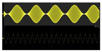
Using hardware-based Zoom technique and record length of up to 1 Gpts, users can select a slower timebase without compromising the sample rate, and then quickly zoom in to focus on the area of interest
