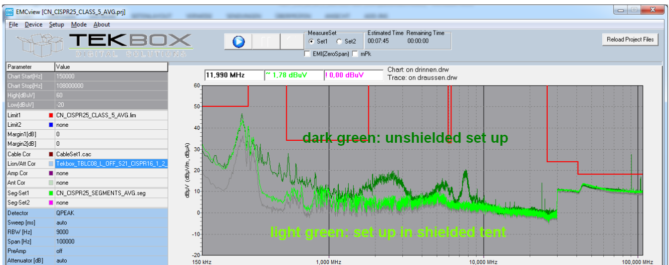
Picture 6: CISPR 25 conducted noise measurement; DUT powered
