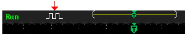
Picture 2-13 signal output of probe compensation
