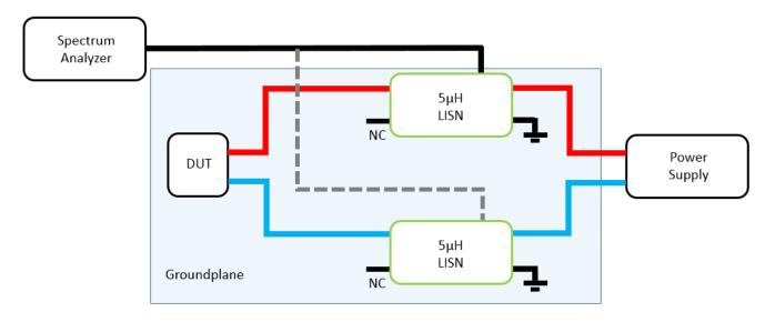
The DUT shall be isolated and elevated from the groundplane. The spectrum analyzer shall measure the conducted emissions on both supply lines. The RF output of the unused LISN shall be terminated with 50 Ohm. If the power return line is less than 200 mm, a set up with a single LISN is sufficient. For the exact details of the set up and for the limits of conducted emissions refer to the CISPR 25 or relevant applicable standard.
