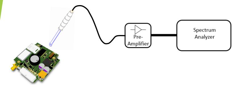
Localize the source of unwanted emissions on the DUT PCB using near field probes and a spectrum analyzer.
